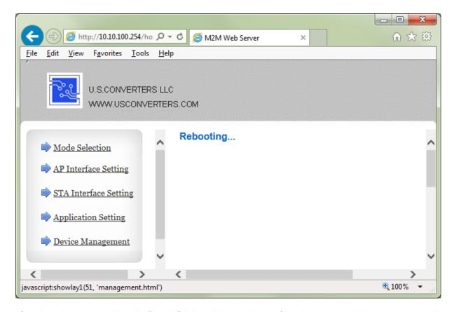
After the reboot is complete the "Ready" light will be steady on. If you have entered the correct network settings and password then the converter will now automatically join the network, and the "Link" light will be on.
