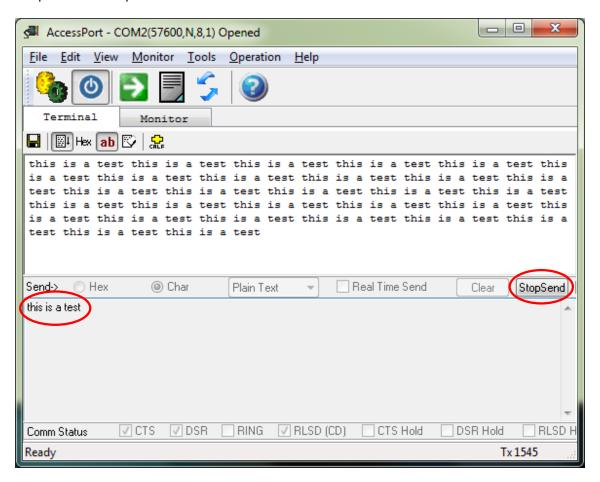
Enter a text string in the lower (send) window in AccessPort and click the AutoSend button. The characters should now be sent via virtual COM 2, over WiFi to the WF5000B module, out on the TX pin, back into the RX pin, back over WiFi, back into virtual COM port 2 and should appear in AccessPorts upper (receive) window.
