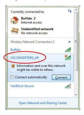
Once your computer is connected successfully to the WF5000B you can open a web browser and enter the WF5000B's IP address which by default is **10.10.100.254**.
