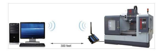
To be able to send programs to your CNC machine over WiFi you will need to connect a Serial to WiFi Converter such as the <u>WF5000B</u> from U.S. Converters LLC to your CNC machine. This will allow you to communicate with your CNC from a PC for up to **300 feet**. As in any regular WiFi network you can use signal repeaters/boosters or Access Points to extend the range.
